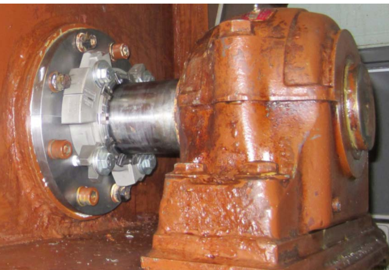
Agitator fitted with a Chesterton 442C Cartridge Split Seal.
