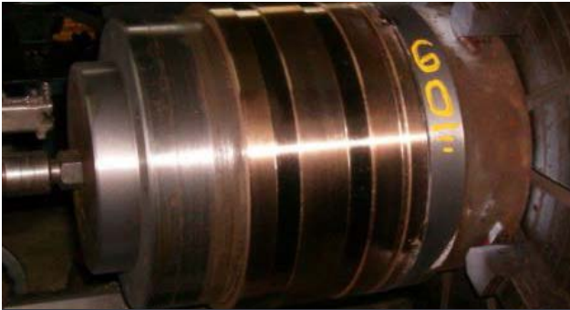
Repair of Hydraulic Jack Ram
